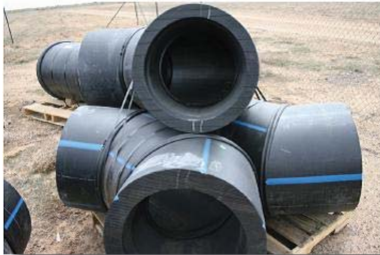
Figure 6.4 Sample fused fittings used for the Eastern Navajo HDPE transmission main
