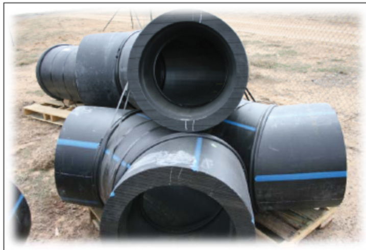
Figure D.6.1 Sample fused fittings used for the Navajo transmission main project
